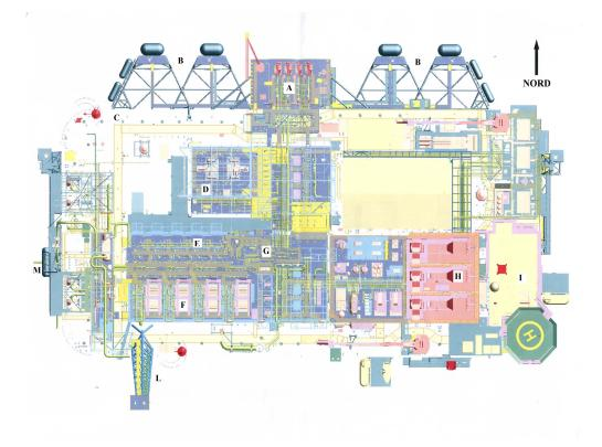
LEGENDA A= Loading Arms B= Fenders C= Tanks **D=** Boil-off gas recover E= High pressure booster pumps **F=** Vaporizers **G=** Waste Heat Recovery H= GTGs **I** = Living quarters L= Flare M= Gas pipeline
